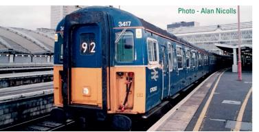
Meanwhile, the 4 VEP (later BR class 423) was designed for semifast/stopping services with 2+3 seating and a door to virtually every seating bay on both sides. The first twenty units (7701-20) were delivered in 1967 and were allocated to the new Bournemouth electric multiple unit depot. It was the ultimate design for commuter traffic, enabling minimum dwell time at stations and very quick coupling and uncoupling in service.
